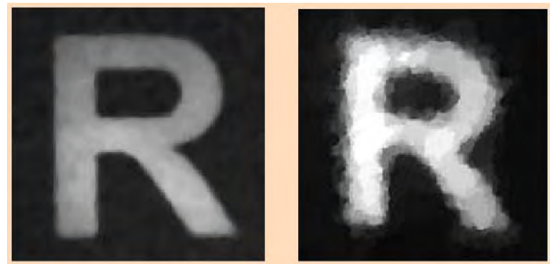
256 × 256 conventional image Single-pixel camera M = 1,300
